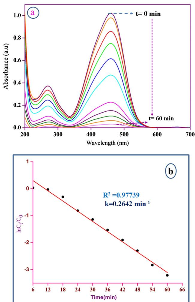
**Fig. 11.** Photocatalytic activity of ZnO NPs (a) plot of absorbance vs. wavelength for the decolorization of methyl orange under UV-light irradiation and (b) its first order kinetics.
