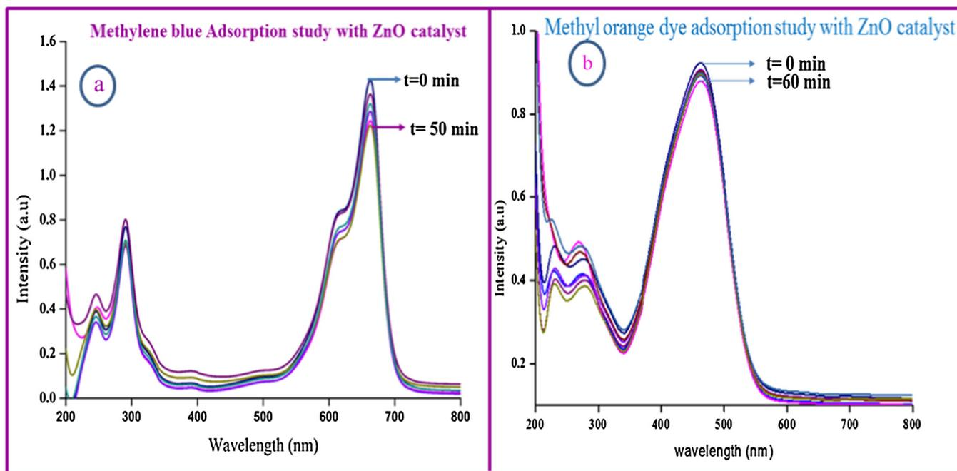
Fig. 8. UV-vis spectra for adsorption kinetics of Dyes by ZnO NPs as adsorbents in the absence of UV light irradiation (a) Methylene blue (MB) and (b) Methyl orange (MO).
