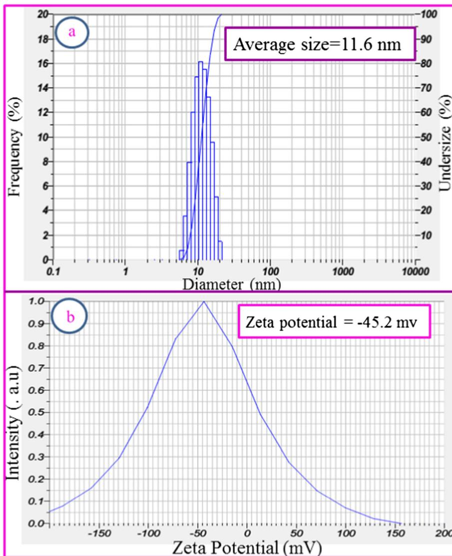
Fig. 5. DLS measurement of (a) average particle size distribution and (b) zeta potential of synthesized ZnO NPs.
