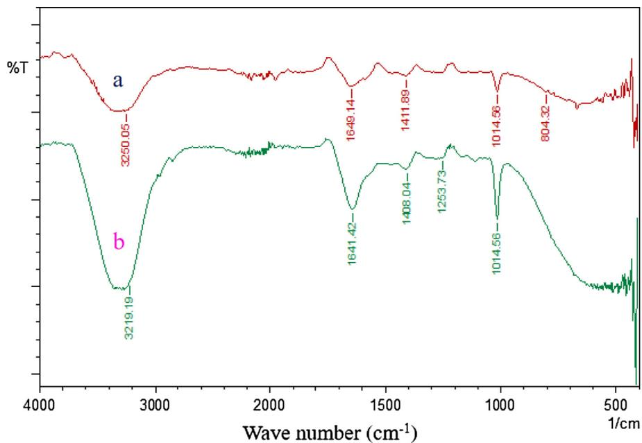
Fig. 6. FT-IR spectra of (a) synthesized ZnO NPs and (b) *Eucalyptus globulus* plant extract.
