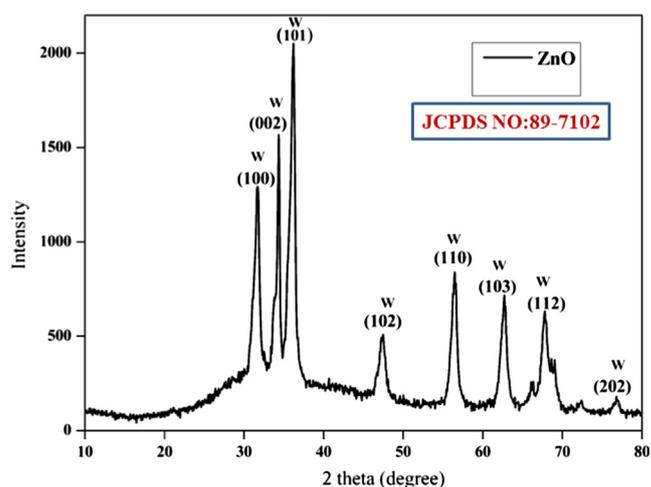
Fig. 2. XRD pattern of synthesized ZnO NPs.
