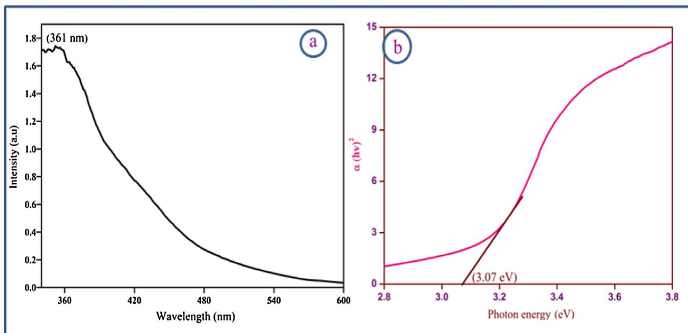
Fig. 1. (a) UV-visible absorption spectra of synthesized ZnO NPs by using *Eucalyptus globulus* plant extract (b) UV-DRS plot of ZnO NPs.
