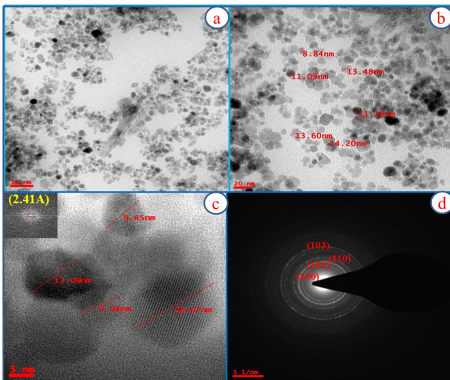
Fig. 4. TEM images of ZnO NPs at different magnifications (a) 50 nm, (b) 20 nm, (c) HR-TEM image of ZnO NPs at 5 nm and (d) SAED pattern of synthesized ZnO NPs.
