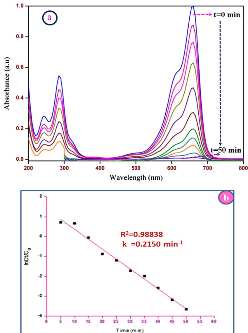
**Fig. 10.** Photocatalytic activity of ZnO NPs (a) plot of absorbance vs. wavelength for the decolorization of methylene blue under UV-light irradiation and (b) its first order kinetics.
