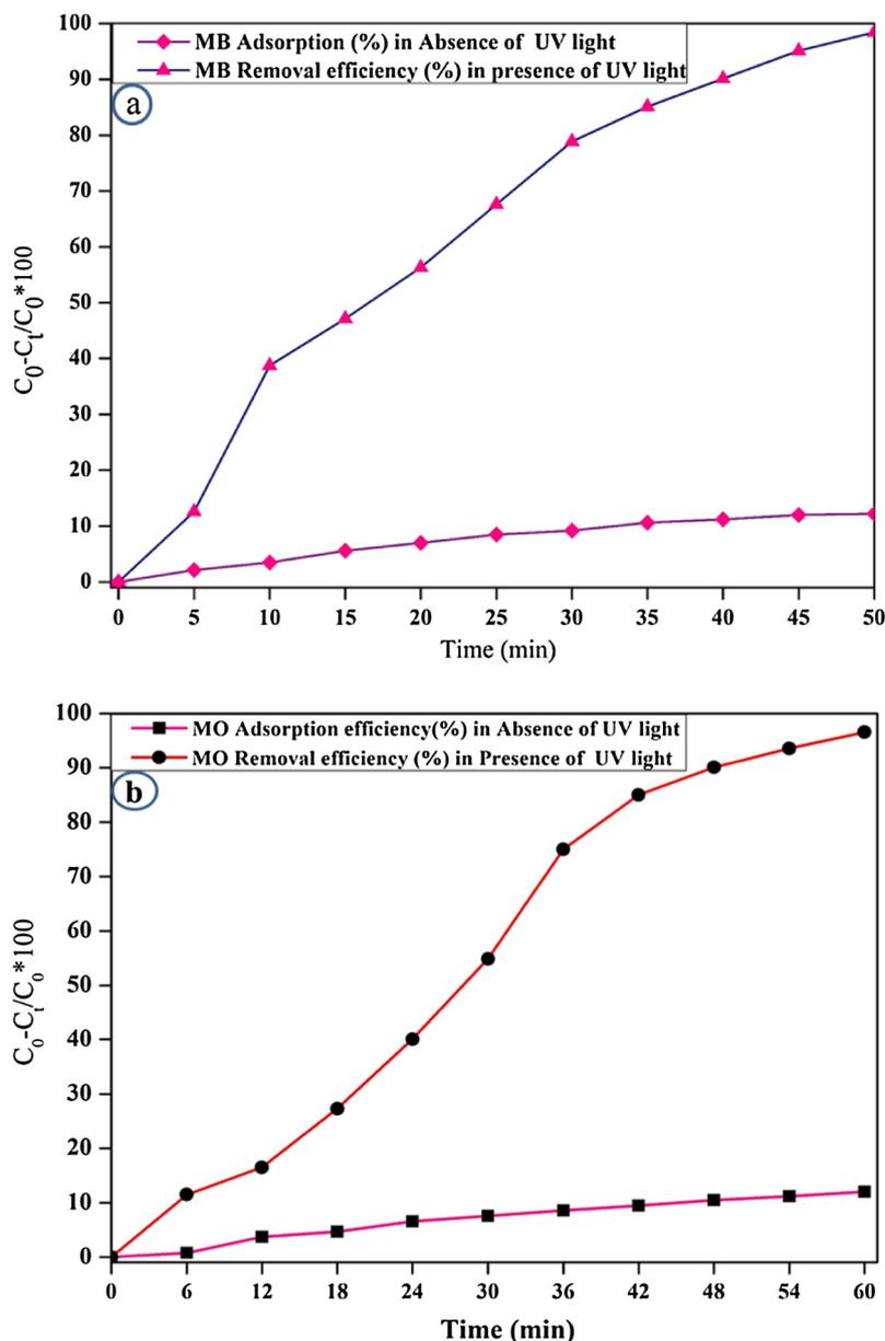
Fig. 9. Removal efficiency (%) of dyes by ZnO NPs as adsorbents (a) MB and (b) MO.
