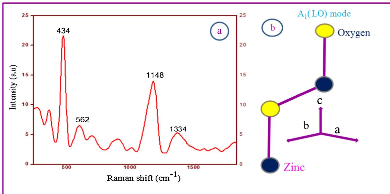
Fig. 7. Raman spectra of (a) synthesized ZnO NPs and (b) longitudinal phonon mode.
