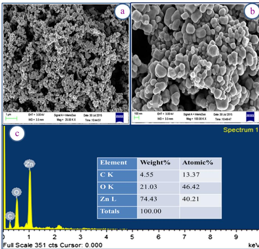
Fig. 3. FE-SEM images of ZnO NPs at different magnifications (a) 1  $\mu\text{m}$  magnification, (b) 100 nm magnification and (c) EDX spectrum of synthesized ZnO NPs.
