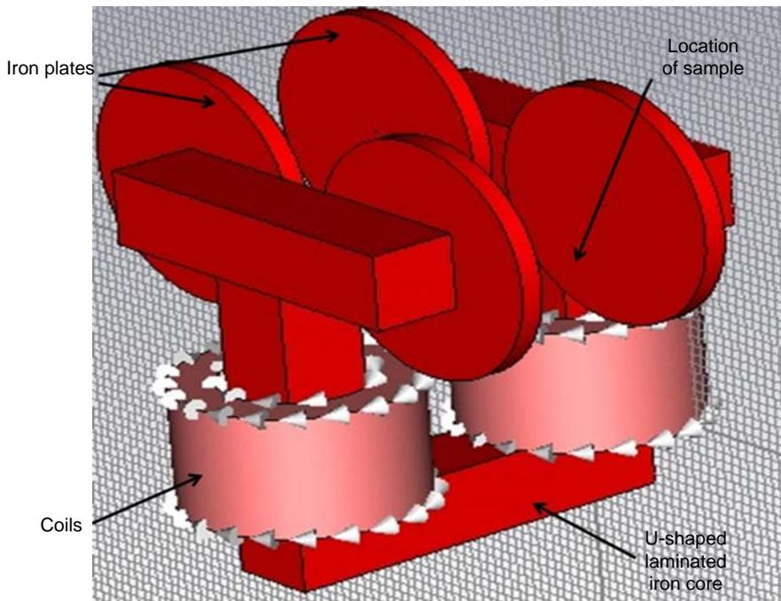
**Figure 1.** Schematic illustration of static magnetic producing apparatus. Coils are wrapped with copper pneumatic tube (not shown). Circulation of water in the tube prevents heating of the samples.
