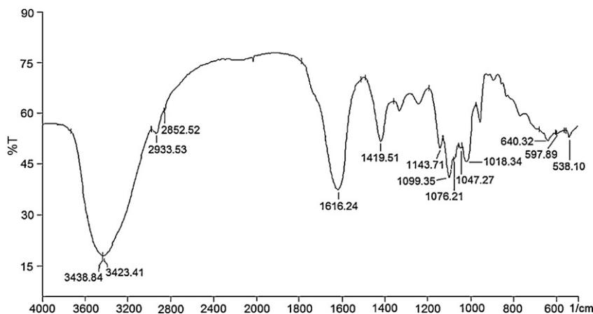
Fig. 1. FT-IR spectra of HCP in the frequency range 4000–500  $\text{cm}^{-1}$ .
