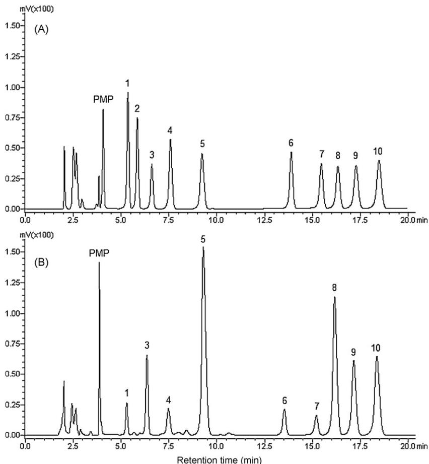
Fig. 2. The HPLC chromatograms of PMP derivatives of 10 standard monosaccharides (A) and component monosaccharides released from HCP (B). The polysaccharide was hydrolyzed with TFA at 100 °C for 8 h and then was labeled with PMP. The HPLC analysis was carried out as described in the experimental section. Peaks: (1) mannose; (2) ribose; (3) rhamnose; (4) glucuronic acid; (5) galacturonic acid; (6) glucose; (7) xylose; (8) galactose; (9) arabinose; and (10) fucose (internal standard).
